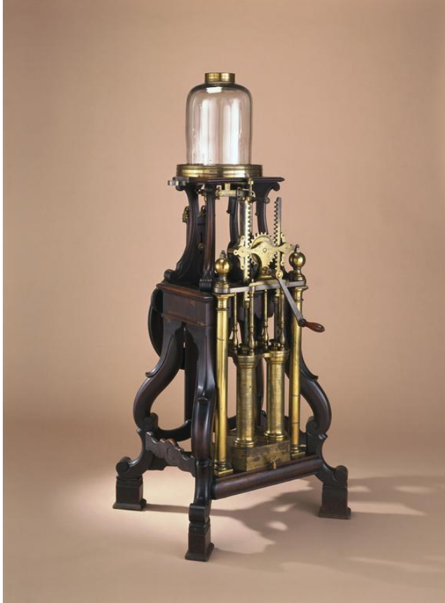
Figure 59 - Science Museum Group. George III's double-barrelled air pump. 1927-1624/1. Science Museum Group Collection Online. Accessed 23 March 2024. https://collection.sciencemuseumgroup.org.uk/objects/co2230/george-iiis-double-barrelled-air-pump-air-pumps-double-barrelled-air-pumps . © The Board of Trustees of the Science Museum, under a CC BY-NC-SA 4.0 Licence.
