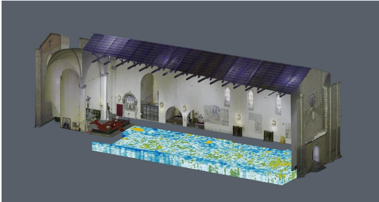
Figure 10. Digital representation in point cloud format of the church of San Domenico (Città di Castello) with the GPR dataset (after Kay et al. 2023: fig. 1, #9).
