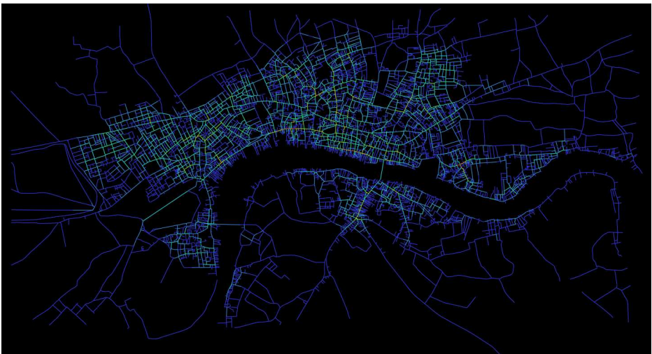
FIGURE 2 Vectorised road networks from Rocque (1746) shown with results of Space Syntax analysis (400 m radius). 'Warmer' colours represent more connected or 'central' locations.
