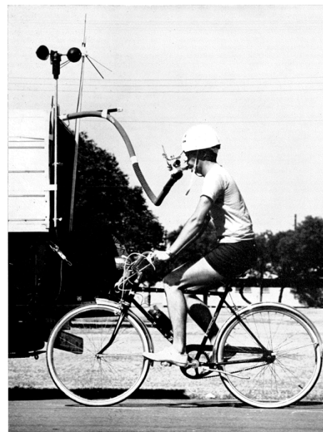
The method used for determining the oxygen cost of cycling measured distance at various speeds.
