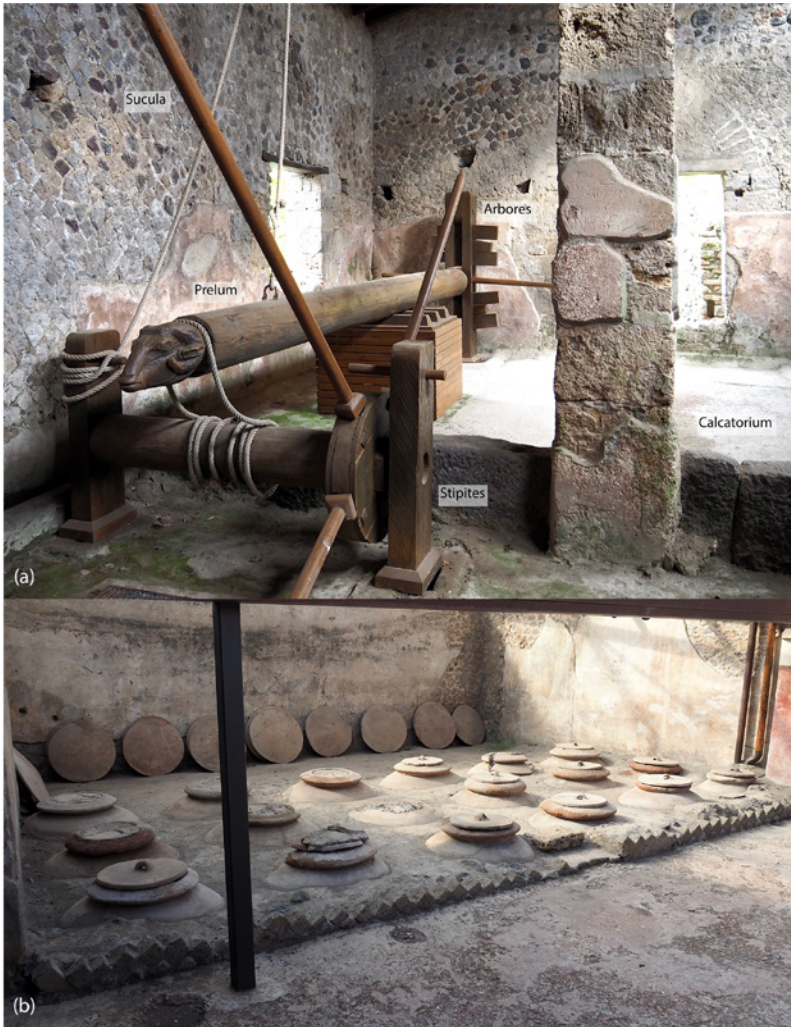
Fig. 3 (a) reconstructed type 1 Roman wine press with structural elements indicated at the Villa dei Misteri, Pompeii, 1 st c. CE (photo by E. Dodd); (b) the semi-open air cella vinaria at Villa Regina, Boscoreale. The double-layer locking dolia lids are preserved on each dolium (photo by E. Dodd)
