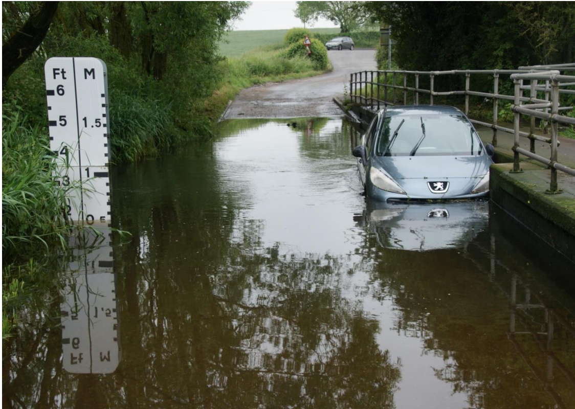
Figure 2.3. Trescott ford, GR SO 852973, June 2019. The Smestow flows from left to right – the car is pinned against the footbridge by the force of the flow, even though the stream depth is shallow and the water is not rapidly moving.
