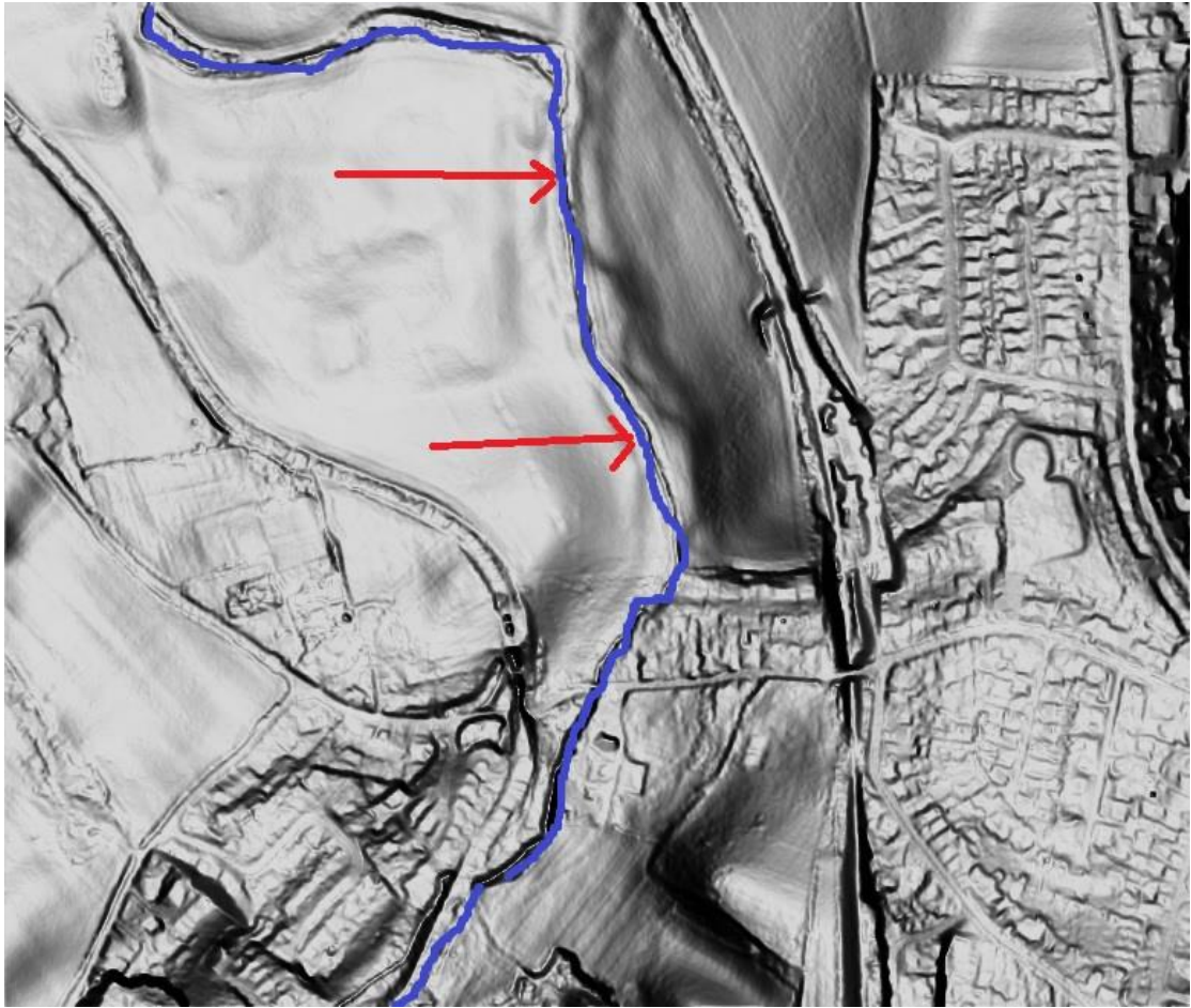
Figure 3.2. LiDAR extract showing an area north of Wombourne with two straight sections (indicated with red arrows) in the course of the Tene brook (blue line). These may represent stream course adjustments associated with a lost mill site. Scale 1:5,000.
